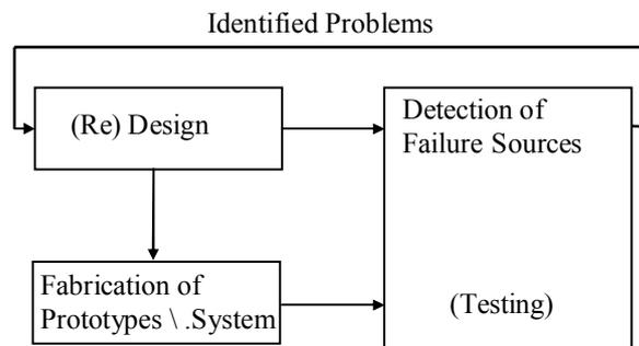
**Figure 2. Reliability Growth Feedback Model with Hardware.**
