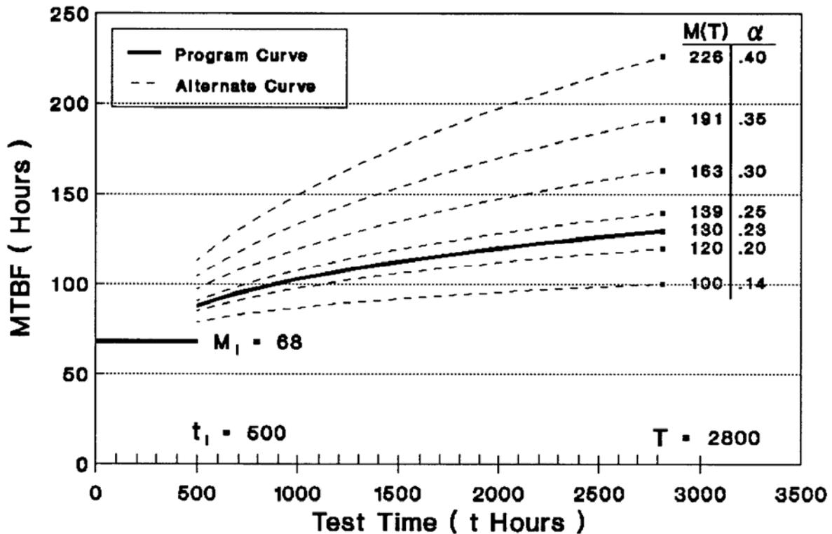
Figure 3. Program and Alternate Idealized Growth Curves.
