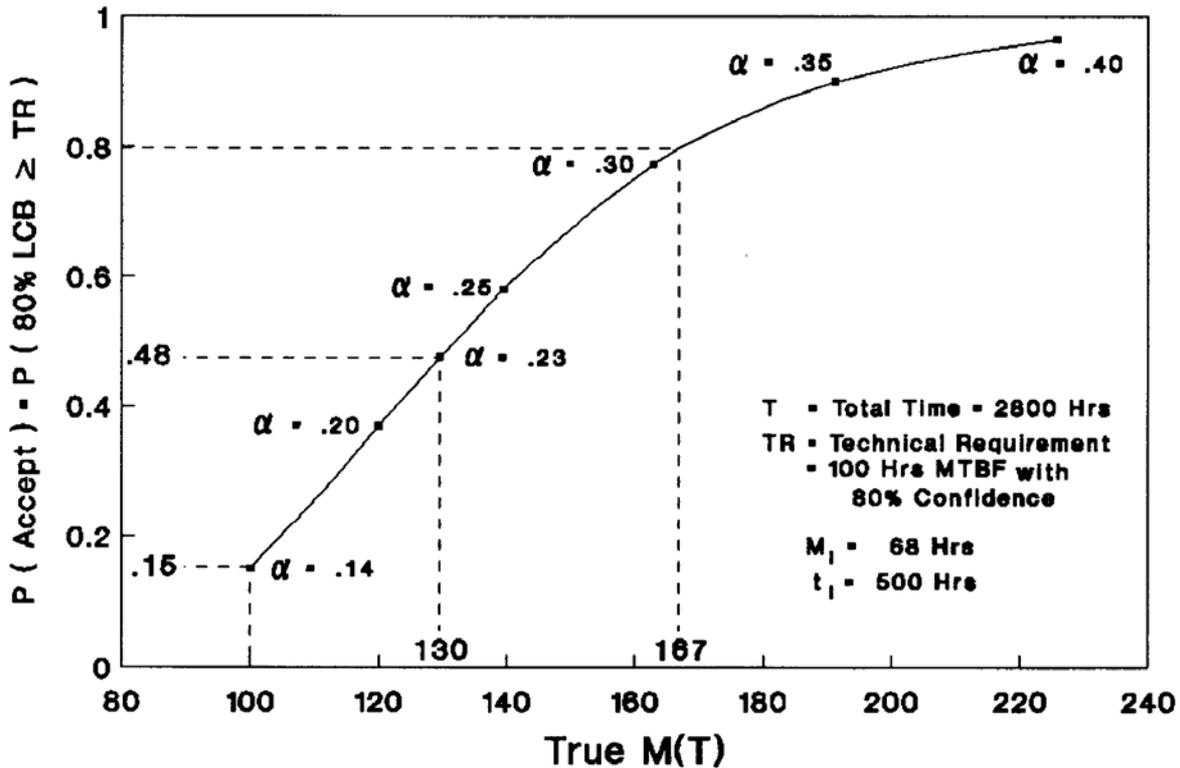
Figure 4. Operating Characteristic (OC) Curve.
