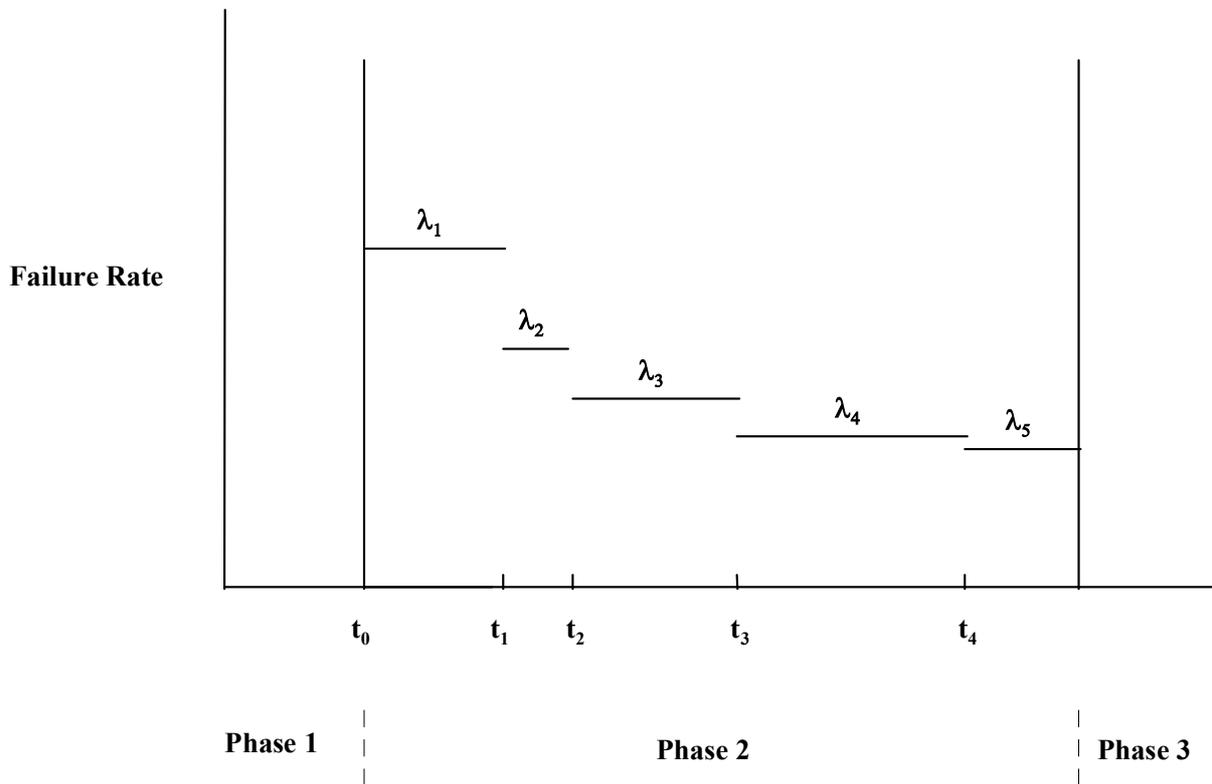
**Figure 3.1 Failure Rates Between Modifications**
