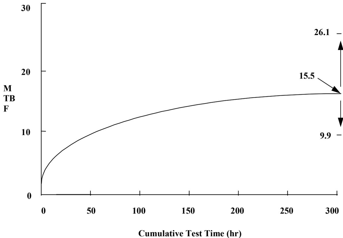
**Figure 3.4.3 Estimated MTBF Function With 90 Percent Interval Estimate at T = 300 Hours**
