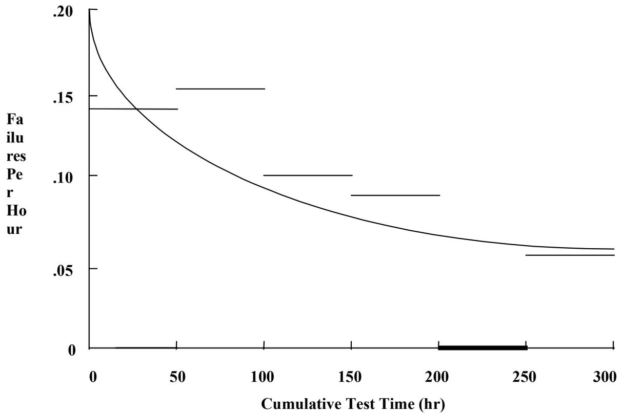
**Figure 3.4.2 Estimated Intensity Function Superimposed On Average Failure Rate Plot From Observed Data**
