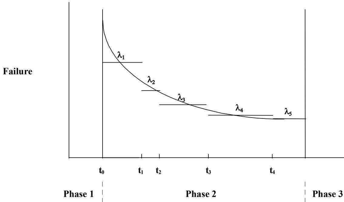
**Figure 3.4 Parametric Approximation to Failure Rates Between Modifications**
