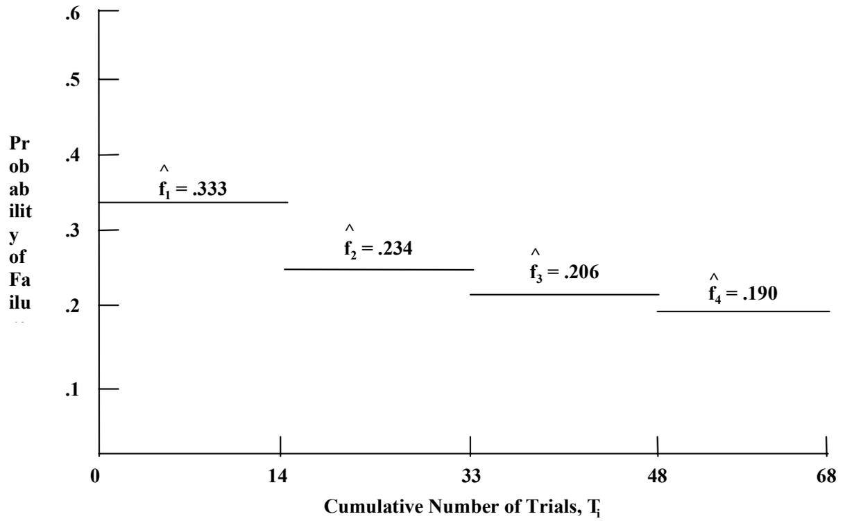
Figure 3.6 Estimated Failure Rate by Configuration
