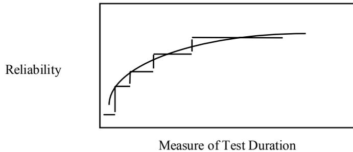
**Figure 6. Graph of Reliability in a Test-Fix-Test Program.**
