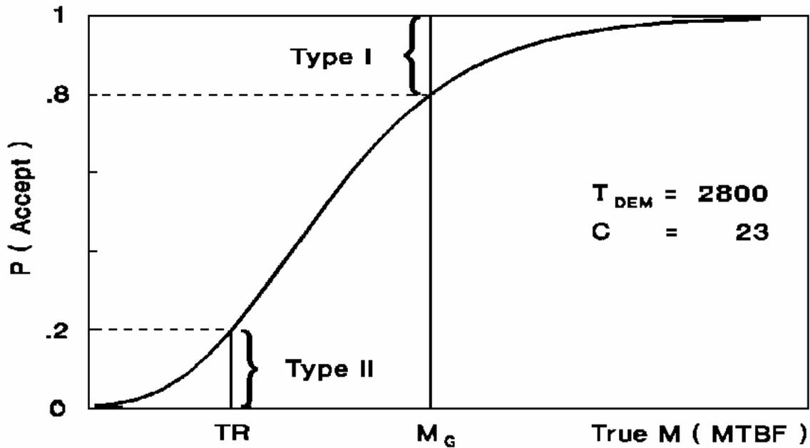
**Figure 1. Example OC Curve for Reliability Demonstration Test.**
