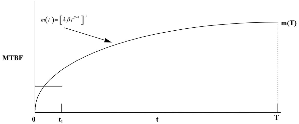
**Figure 3.4.1 Test Phase Reliability Growth Based on AMSAA Continuous Tracking Model**
